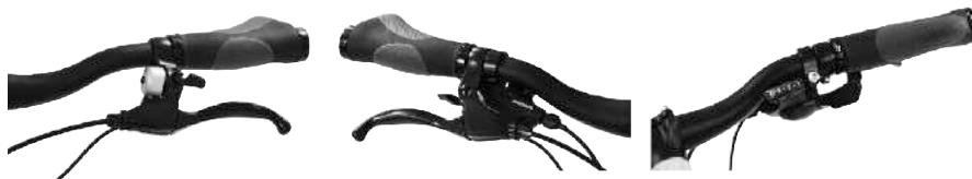
When braking hard by pulling the brake levers towards the handle bars, you should not push the braking force to its upper limit. Or, the braking distance will be extended and there is a risk of accident. Adjust the brake levers as mentioned above.
